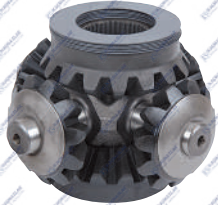
1522343 Spider 1 pc + 1522348 Side Gear 2 pcs + 1522346 Side Pinion 4 pcs + 1524716 Thrust Washer 6 pcs + 1522347 Thrust Washer 4 pcs + 1522345 Needle 140 pcs + 1522344 Spacer Plate 4 pcs
